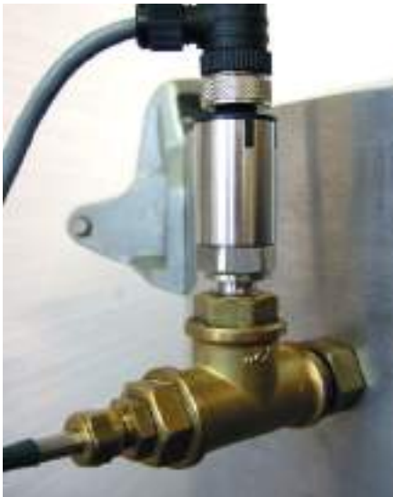
The pressure and temperature sensors continuously measure the conditions in the autoclave.
