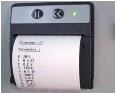
The programming parameters, temperature and pressure curves, and key data are printed at the end of sterilization, ensuring traceability of your process.
